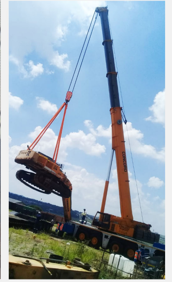
Lifting 50Ton mobile Crusher
